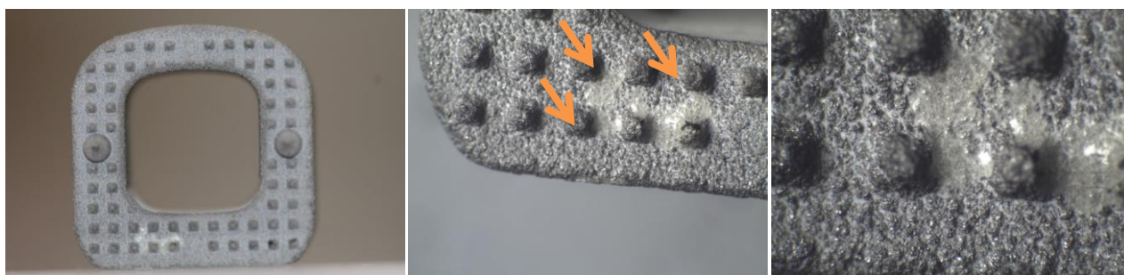
Fig 1. Day 7 Ti-PEEK Photographs TES-10: There is a deposit on this sample that is clear in color and the entire endplate surface showed signs of white accumulation.
